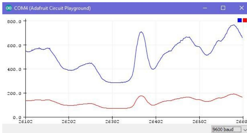
Hey, the text we added doesn't even show up, but the plotted number ranges do! Now you can really visualize how mapping changes your sensor values. The blue line is what the sensor is reading, and the red line is the new mapped value that we can send to an analog LED to make it dim or brighten according to what the sensor senses.
