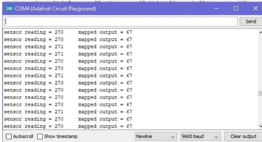
Here we take the large range of **0** to **1023** and smoosh it down to the range of an analog LED, that of **0** to **255**. See how the mapped output is a much smaller range than what the sensor reading actually is?
